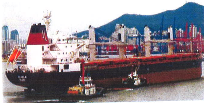
M/V Charlie, a 34,168 MT DWT newbuilding bulk carrier equipped with 4 cranes of 36MT
